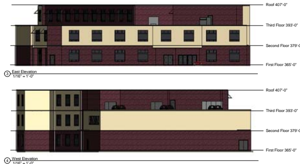
Figure 3 displays the East facade of the school building. The doors seen on the first floor are for emergency exit only. The door seen on the third floor leading to the roof is for access to perform maintenance on the mechanical equipment.
